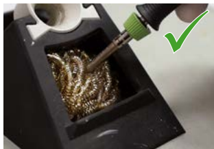
Just stick soldering tip into dry cleaner and turn
