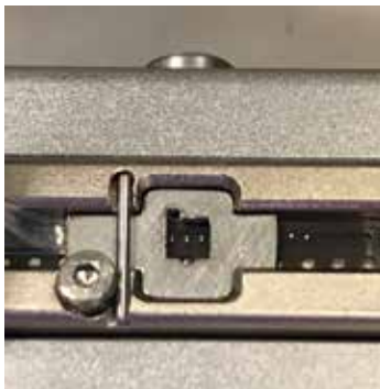
Provision of 01005 components with a tape feeder
