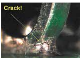
Lead-free PLCC: micro crack
