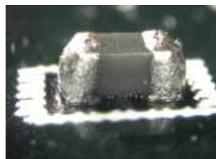
0402: bulbous solder joint
