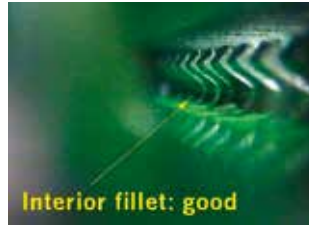
PLCC – interior fillet inspection
