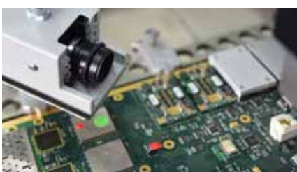
Live process monitoring on the HR 600 XL
