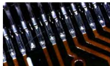
QFP solder joints – taken with the Erska MOBILE SCOPE MACROZOOM optical head
