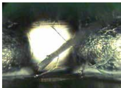
BGA: contamination (fibre)
