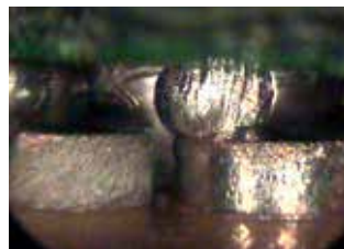
BGA – piggy back: bad alignment
