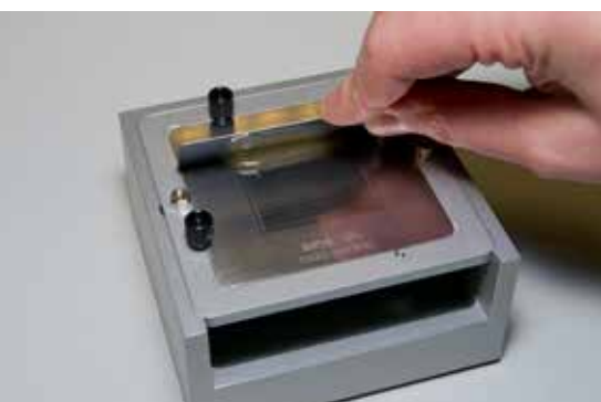
Flux deposition in the dip stencil
