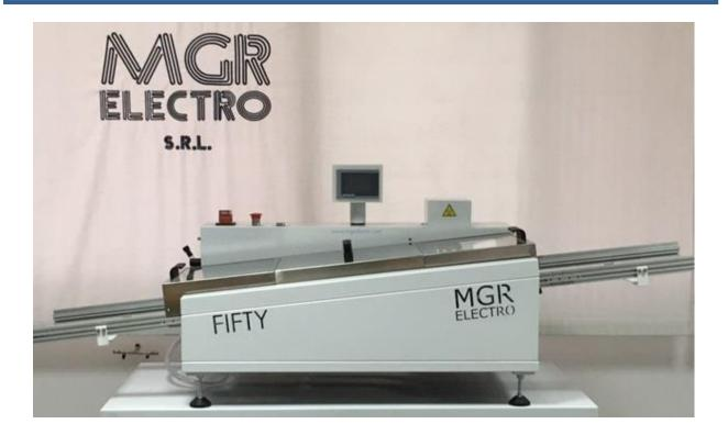
FIFTY soldering machine has been created by MGR ELECTRO to be used for the soldering of electronic components on printed circuit boards with PTH/SMD technology both for lead containing and lead-free alloys.
