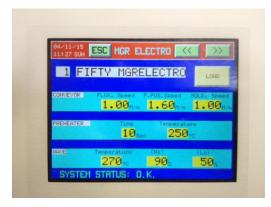
FIFTY is managed by a very practical PLC through which you can set any parameter of the machine. This PLC may recall up to 20 stored programs.
