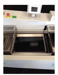
Preheating is performed by an IR panel protected by a PYREX glass and through the PLC the circuit board to be soldered can be stationary in the preheating zone for up to 90 seconds or run in continuous mode for faster production.
