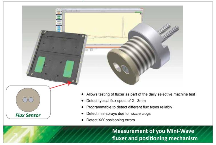
After discussions with both customers and machine manufacturers, the main problems reported in fluxing within the selective process was X/Y positioning problems and crystallisation/nozzle clogging. These two issues often result in flux being deposited in the wrong areas on an electronic assembly, insufficient fluxing of necessary components will result in poor soldering quality, and potentially un-activated flux could seep under sensitive electronics, producing in-field issues.
