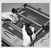
Removing excess solder with hot air and de-solder braid.
